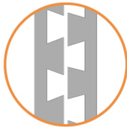
VANE thread design
